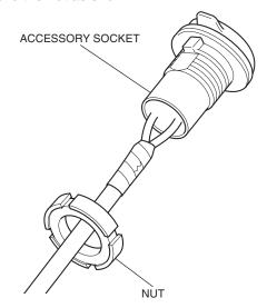
8. Remove the dummy connector as shown. <Left side>
