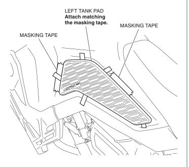
5. Remove the adhesive backing as shown.
