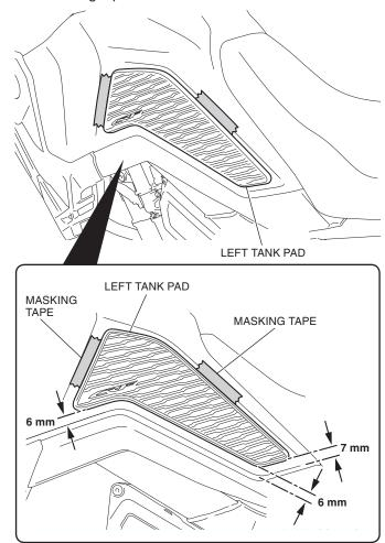
3. Peel off the adhesive backing on the left tank pad as shown.
