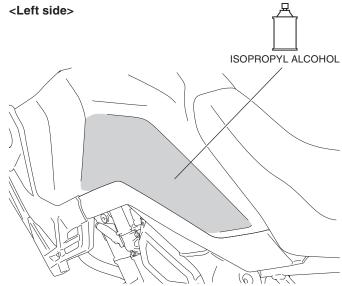
2. Arrange the left tank pad as shown and mark with masking tape.
