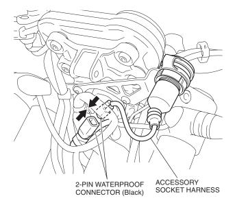
18. Secure the accessory socket harness with the wire tie as shown.
