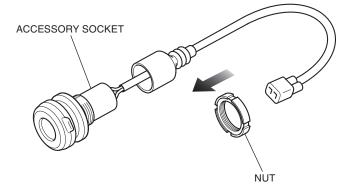
10. Assemble the accessory socket as shown.
